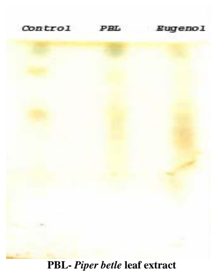
Figure 2. TLC profile of the phenol extracts from the castor leaves surface treated with two allelochemicals (24 hrs after exposure to P. betle and eugenol).
